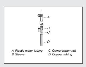
5. Using an adjustable wrench, hold the nut on the plastic water line to keep it from moving. Then, with a second wrench, turn the compression nut on the copper tubing counterclockwise to completely tighten.
